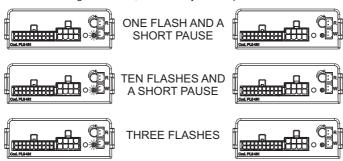
Press the remote controls lock/unlock buttons to make sure the alarm system works properly. Eventually disconnect the 20-way connector and reconnect it after few seconds.
